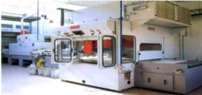
UV Spray application system with UV curing chamber seen at end. Picture courtesy of Burkle Process Technology Loerrach Germany
