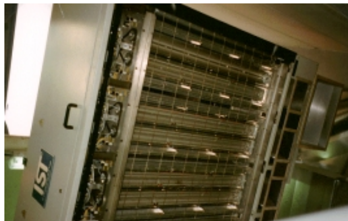
Shown is a 60 inch 3 bulb system with shutters following immediately after the spray application booth. Picture courtesy of IST Metz - USA
