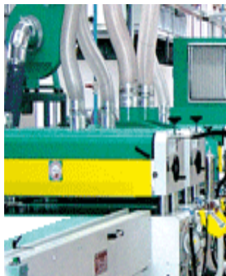
The 4 foot by 8 foot vertical grain Douglas fir veneer panels move through the 60 foot long UV curing line in about two min.
